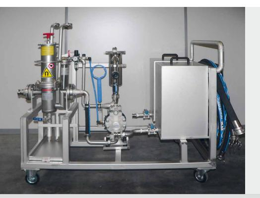
Separation of smallest, magnetic residues and filtration of aqueous cleaning media.
